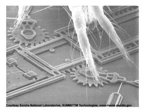
Figure 1. Spider mite with legs on a mirror drive assembly, illustrating the tininess of nanotechnology. *Credit*: Sandia National Laboratories, SUMMiTTM Technologies, http://mems.sandia.gov/scripts/images.asp
